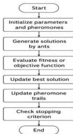
Figure 1. Process Ant Colony Optimization Method
