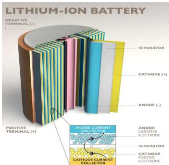
Figure 3. Lithium-ion Battery Construction
